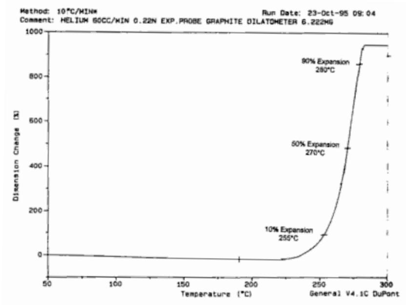
Figure 4: Thermomechanical Analysis (TMA) Plot for GP2 Intumescent Resin
