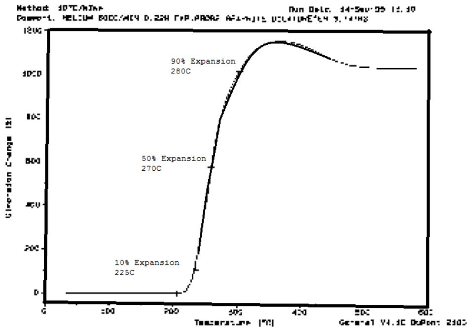
Figure 3: Thermomechanical Analysis (TMA) Plot for GRAFGUARD™ Grade 373
