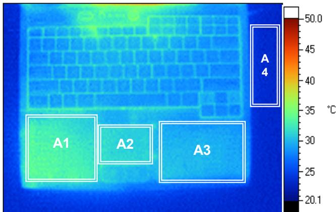
Fig. 9. Thermal image of the laptop cover and keyboard taken with the 0.51 mm 369 W/mK graphite spreader in place
