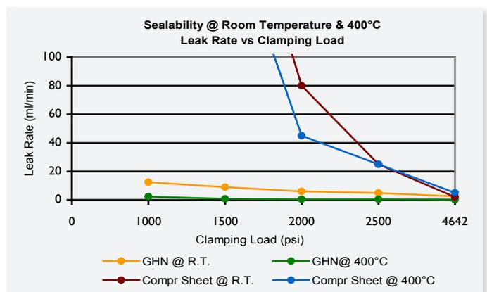
While maintaining an effective seal, GRAFOIL® material exhibits virtually no creep relaxation. As a result, the need for periodic bolt tightening is greatly reduced.
